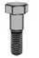
DIN 7999 - 1983 High strength hexagon fit bolts with large width across flats for structural steel bolting
